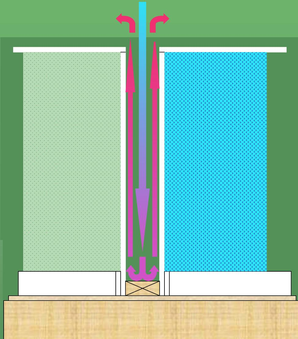
Given an open topped wall (common in balloon construction or at the party wall in a split level), cold attic air will drop down the center of the wall cavity to the bottom & then rise up the sides being warmed as it goes back to the attic.
