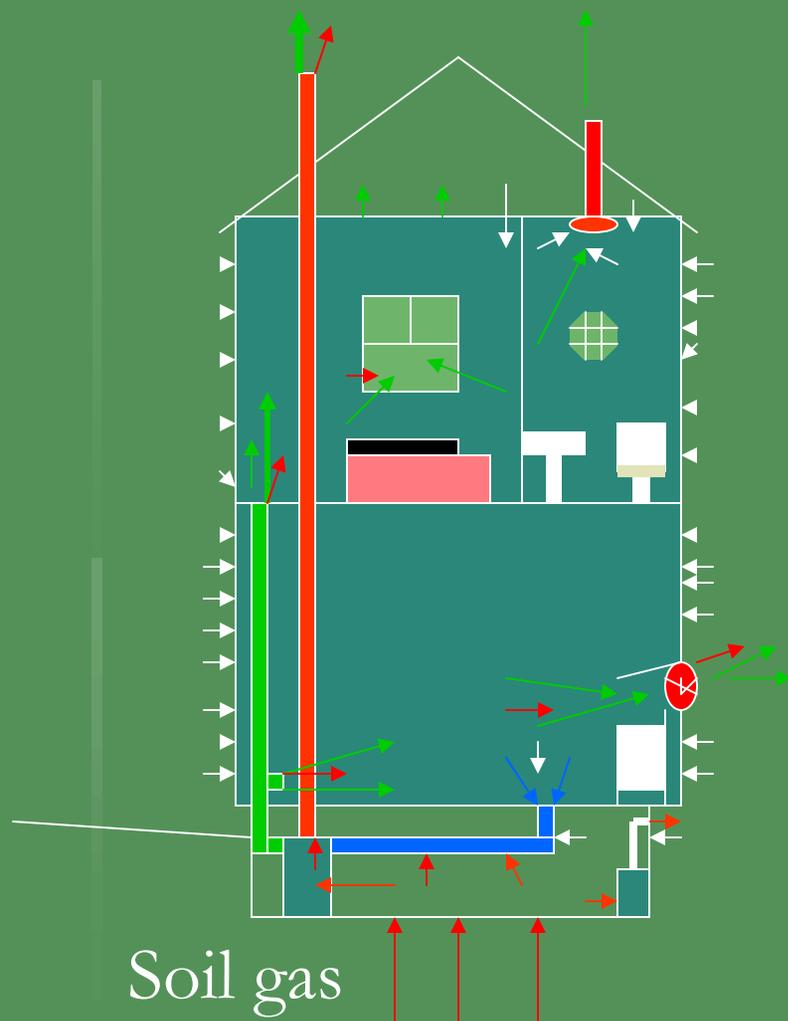
The ducts on a warm air heating system add another variable:
