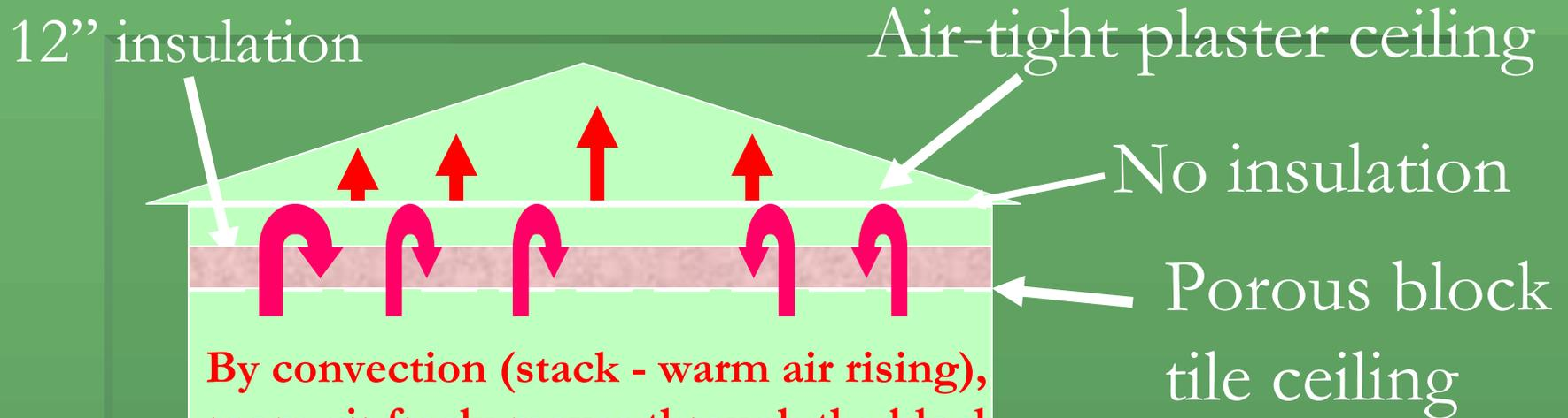
By convection (stack - warm air rising), room air freely moves through the block tile & insulation, warming the area between the ceilings to the same temperature as the room below.
