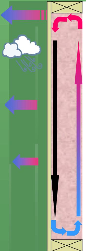
Air inside a wall cavity moves up the heated side picking up heat. It then drops down the cold side, depositing heat which is in turn conducted to the exterior.
