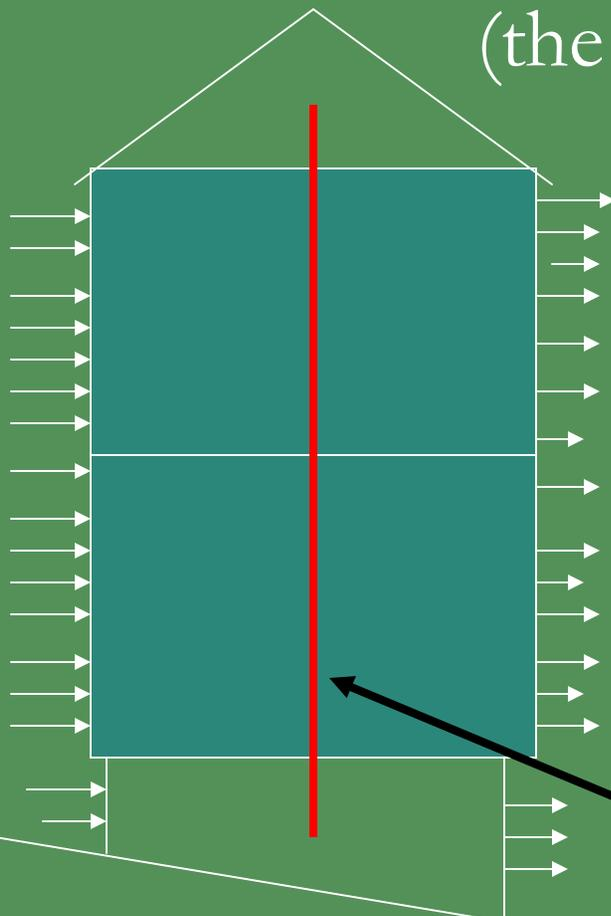
Wind blowing against the building pushes air in the windward side and sucks it out the leeward side.
