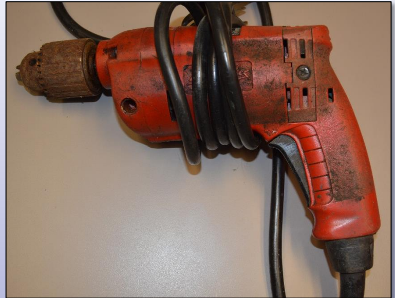
A Milwaukee Drill for drilling holes for wall insulation
